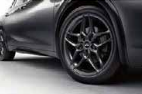
19" LIGHT ALLOY WHEELS WITH 5 DOUBLE-SPOKES, 235/45R19 RUN FLAT TYRES STANDARD ON Q30 SPORT AND SPORT PREMIUM
