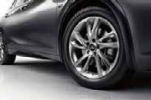
18" LIGHT ALLOY WHEELS WITH 5 DOUBLE-SPOKES, 235/50R18 TYRES STANDARD ON Q30 GT
